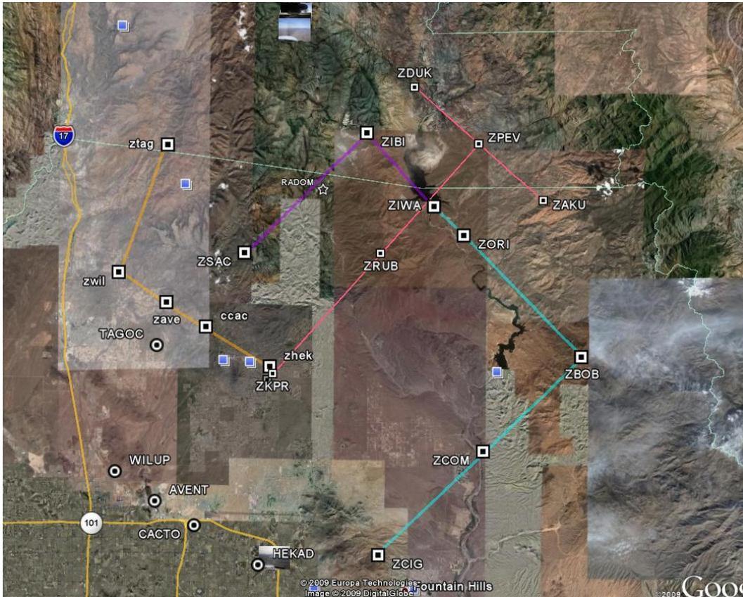
**STEP 4** Print the spreadsheet page showing the offset approach and take it to the airplane. Enter the offset waypoints into the User Waypoint menu. Then create a flight plan for each offset approach. Manually set the CDI sensitivity manually to 1 nm before you arrive at the IAF and then to .3 nm just before that FAF. Otherwise it will fly the same as the actual approach. The picture to the right is the GPS track of a student flying the KSDL GPS D offset approach.
